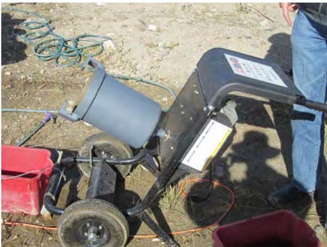
3) Grind up to 1 kg (2.24 lbs.) of tabled concentrate with 50% water and 40% rod volume for 6-10 minutes at 72 rpm in a 200 mm (8" diameter by 12") rod mill.
