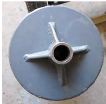
Note: This rod mill is 200 mm (8") inside diameter and 300 mm (12") long inside the mill.
