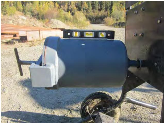
*Note: Loading the rod mill with concentrate & rods & water in the vertical position*
