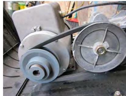
Note: The original pulleys need to be changed from a 6" to a 4.5" on the gearbox and from 1.75" to a 4" diameter adjustable pulley on the motor to increase the speed from 25 rpm to 72 rpm (for 200 mm, 8") rod mills.
