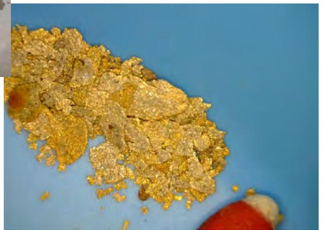
*Gold before and after grinding at low solids loads in a rod mill.*
