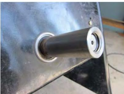
Note: This is a close up of the 24 mm metric female adaptor which screws onto the horizontal drive of the MultiQuip MixNGo Model MC3PEA two cubic foot portable cement mixer. It has to be machined. The threaded end is welded onto the back of the rod mill as shown in the center photo.
